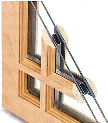
Paired with SDL bars on the exterior of the glass, a spacer bar is installed between the glass, creating an even closer match to the Authentic Divided Lite look.
